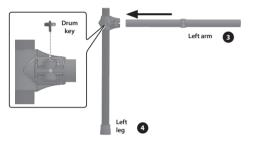
1-2. Once the pipe is fully inserted, firmly tighten the bolt with the drum key
