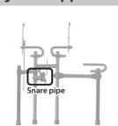
**3–1.** Use the drum key to loosen the bolt of holder C, and insert the snare pipe **9** into holder C of the center frame
