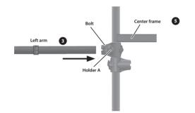
**2–2.** Once the pipe is fully inserted, firmly tighten the bolt with the drum key.
