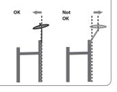
\* When attaching the PDX-8 (snare), refer to "About the memory clamp" on the other side
