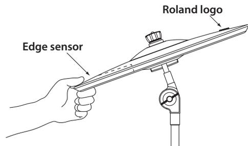
\* When ONLY using the BELL output of the CY-13R, the choke function will not work.
