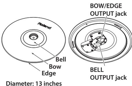
\* The CY-13R is not capable of detecting the striking position. If you're using a Roland percussion sound module that is capable of detecting the striking position, you'll need to set the ride's Position Ctrl to OFF. For details on how to make the setting, refer to the owner's manual that came with your percussion sound module.
